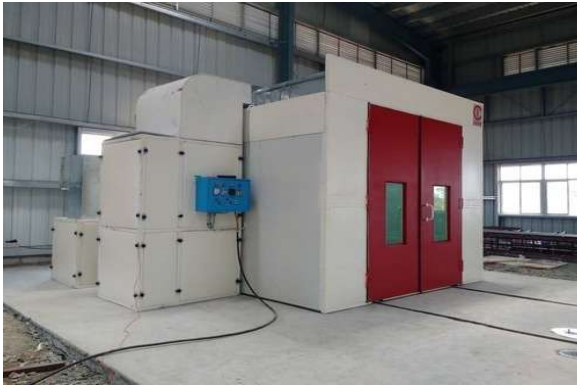
Spray Paint Booth
